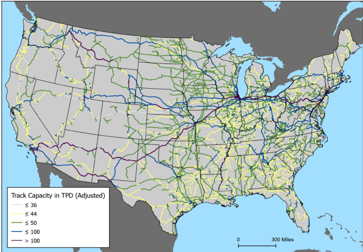
Figure 9. Track Capacity *after* Adjustment<sup>44</sup>
